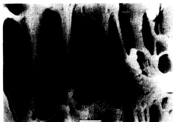
Figure 7 Cavitation of two rubber particles in a rubber-modified polyamide 66 recorded from the stress-whitened zone of TENS1 view of sample 98-2 after uniaxial tensile test. The scale bar represents 2 \mu\text{m}
