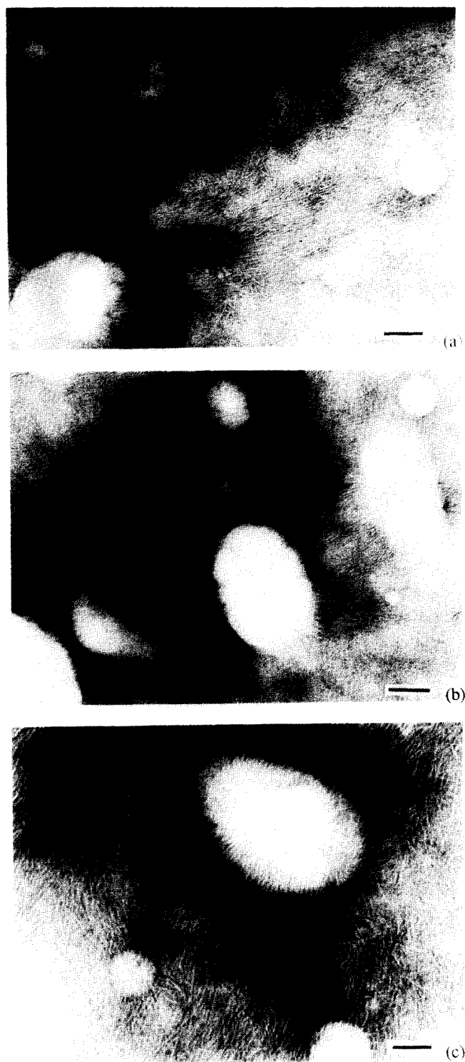
Figure 2 TEM micrographs of different regions in a polyamide 6 modified with EPDR- g -MA: (a) and (b) are taken at low magnification and (c) at high magnification. The sample was negatively stained with phosphotungstic acid. The dark lines are the amorphous regions and the white lines are the lamellae. The rubber particles are not stained and appear white. The scale bars represent 200 nm in (a) and (b) and 100 nm in (c)
