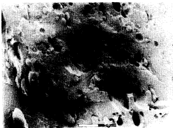
Figure 8 Debonding of rubber particles from the polyamide 66 matrix in sample 98-1 with no grafting agent. The scale bar represents 50 \mu\text{m}
